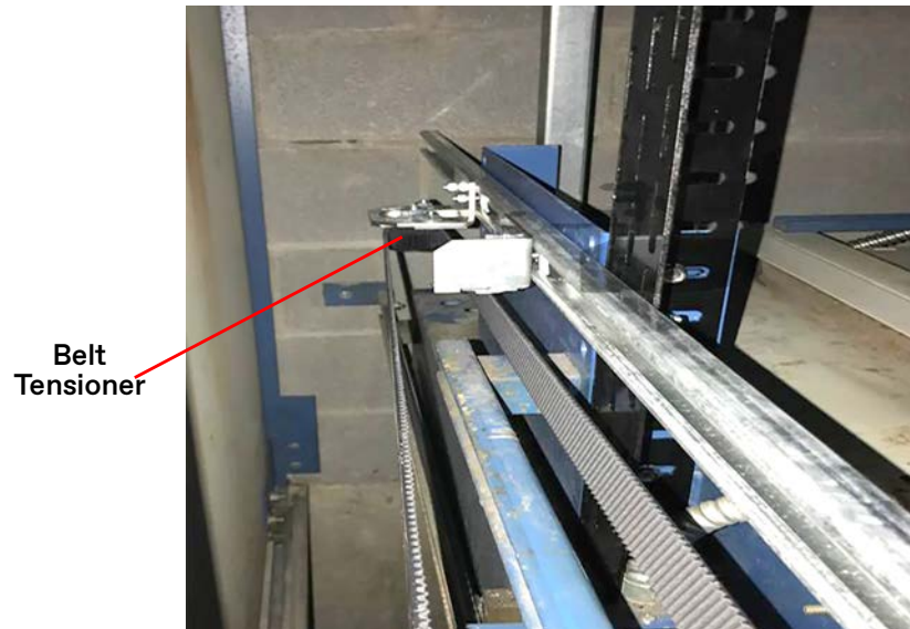
Figure 8 - Belt Tensioner Installation
