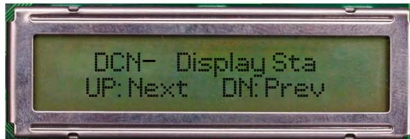
6. **CN Node = 0** displays. Press **UP** or **DOWN** to select the proper CAN Node ID, and press **ENTER**.
