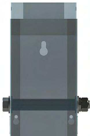
Install strain bolt in the wireway as shown. Remove one knockout on each side of the wireway and install the strain bolt. Secure hoistway wires to the bolt with tie wraps.
