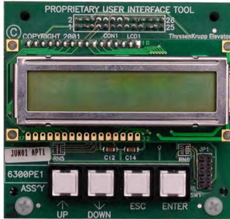
Requirements when replacing an OST (Owner's Service Tool)
