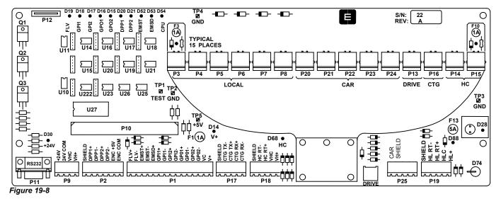
+5VDC SPU supply (+5V TP5 should read between +5 to +5.1 VDC), and a special "TEST" (TP1) used in conjunction with some Human Interface commands to monitor SPU operation.
