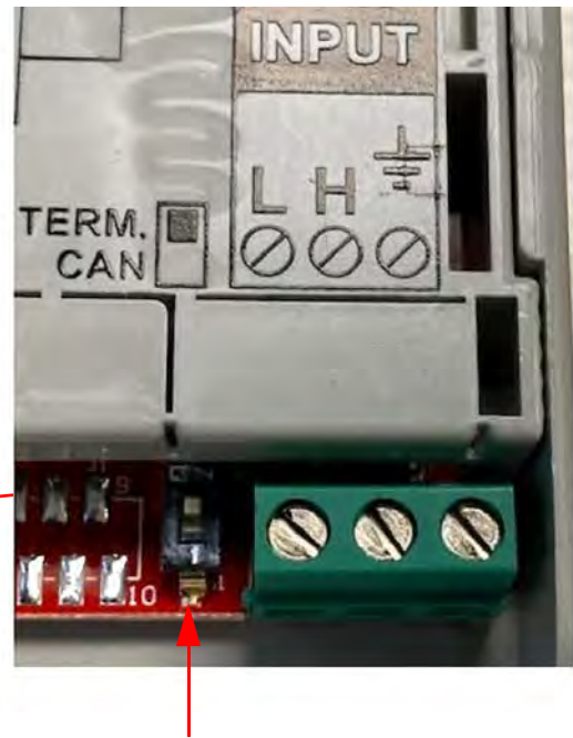
CAN Termination Dip Switch
